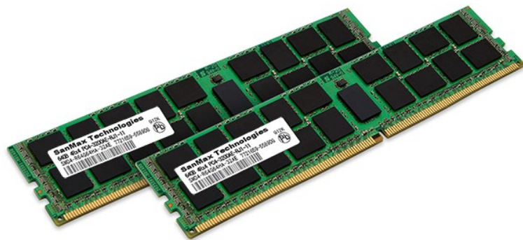
DIMM (Dual Inline Memory Module)
